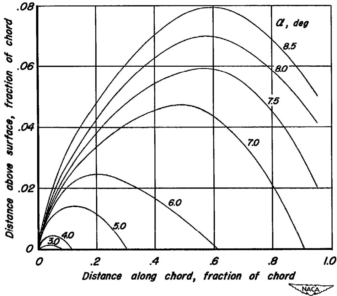
Figure 4.- The extent of upper-surface flow separation on a faired double-wedge airfoil section (ref. 4).
